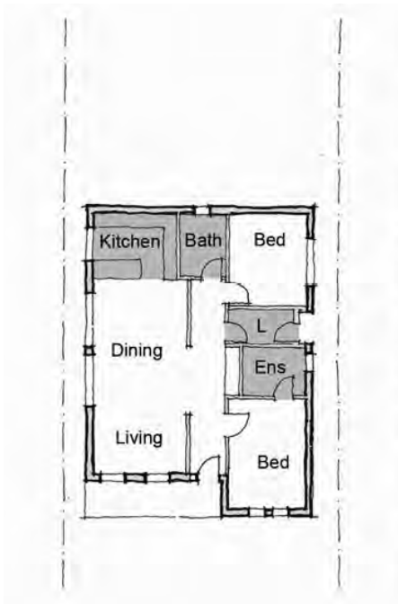
A typical house plan (above) often requires the expensive relocation of wet areas such as bathrooms and kitchen if the house is to be extended.
